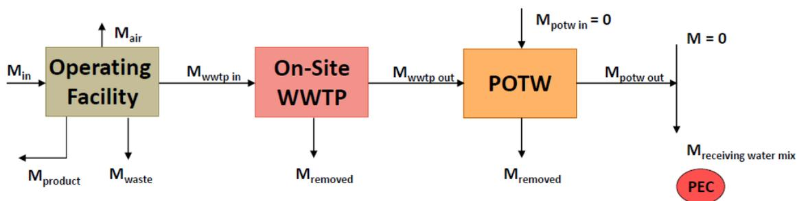
Figure 4 PEC calculation based on API loss in aqueous waste
